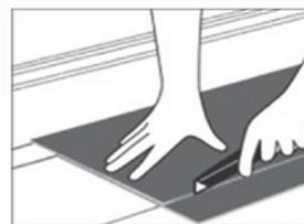
cutting line where the planks overlay. Check that the cut plank fits correctly. Then spot glue or tape all the planks in the last row and press into place. The plank should not be forced into place.
