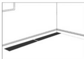
**Note:** For heavy-duty commercial applications, or areas with excess moisture (bathrooms, laundry rooms, restaurants, etc.), the planks must be permanently glued down.
