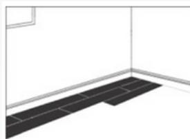
above. To fit air vents, door frames etc., make a cardboard pattern as a guide and use this to draw an outline on the plank. Cut to shape and check that it fits. It should fit snugly and should not be forced into place.
